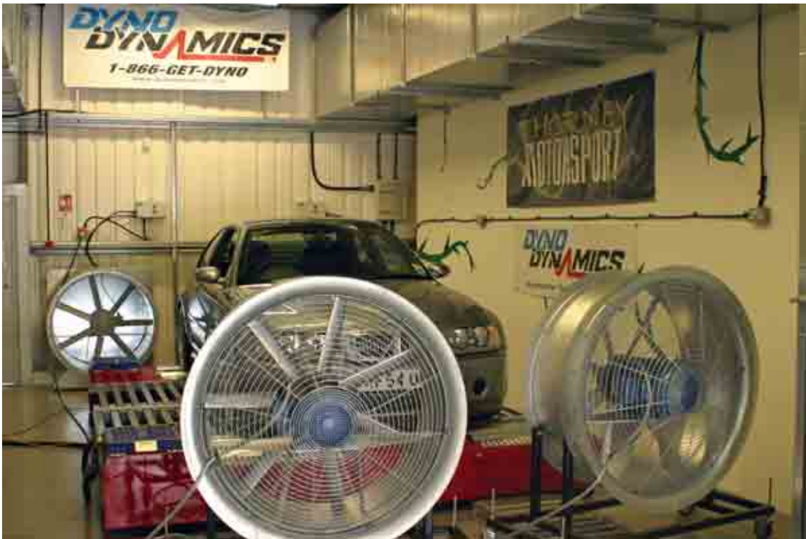
The Thorney Motorsport dyno cell, showing the 1m radial fans.
