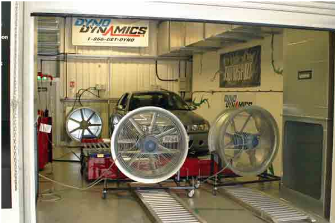
The Thorney Motorsport dyno cell, showing the Dyno Dynamics chassis dyno.
